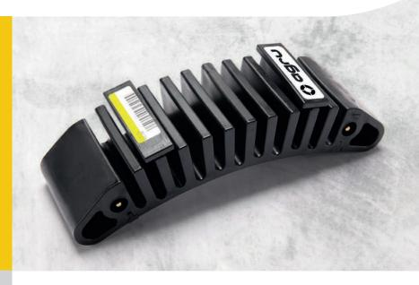
The AGRU Flex Restraint is a flexible bar for electro-socket welding onto PE 100 / PE 100-RC pressure pipes. This way, a rigid system by fixed points can be created that absorbs high forces to prevent axial movement.
